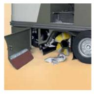
The pressure and height adjustment of the central brush are controlled simply by the knob near the brush. Brush height adjustment depending on wear can, therefore, be done very easily. This ensures a longer brush life cycle
